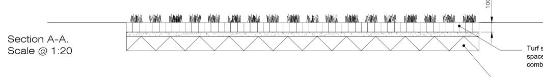
D 01 Drawing LD-05-PP Turf stone grass paving system to parking bays Scale @ 1:20
