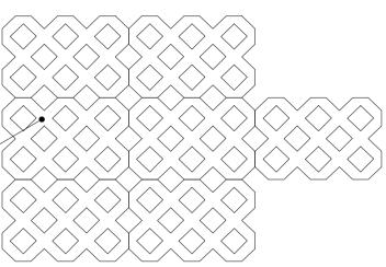
Turf stone grass paving system for parking \_\_ spaces. With 600x400x100mm with Honey combed cavities to facilitate grass growth
